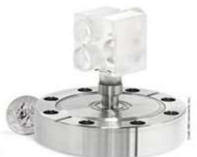
At the heart of a new NIST portable pressure sensor is a dual cavity for laser measurements that is only 2.5 cm long.
