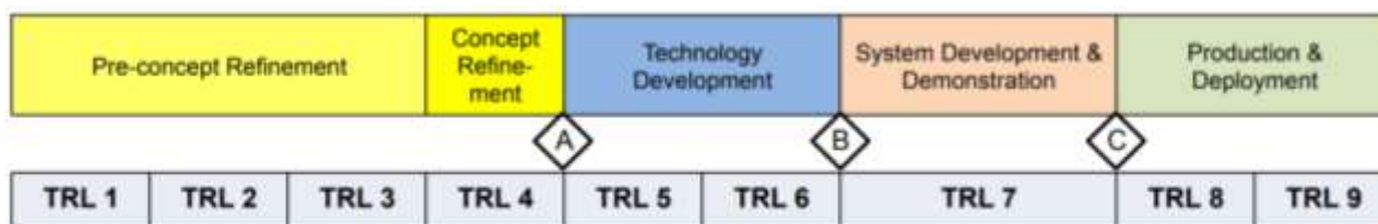
Figure 1: Mapping of technology readiness levels to US Department of Defense System Acquisition Process. Technologies are expected to achieve TRL 4 by milestone A, TRL 6 by milestone B, and TRL 7 by milestone C.
